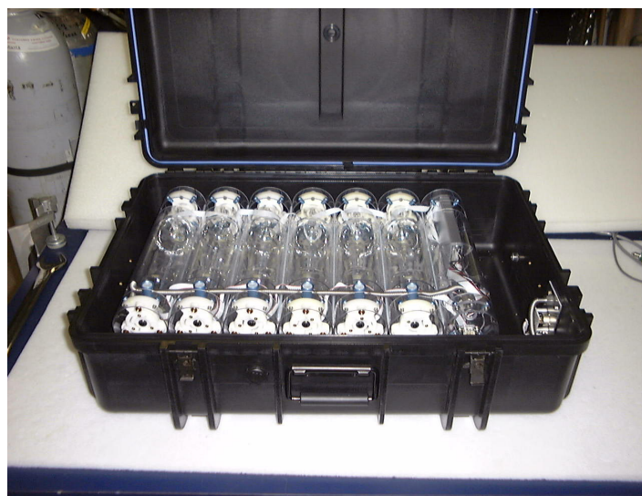
Fig. 4-2: Programmable Flask Package. It has two layers of six glass flasks with motorized valves, a stainless steel gas manifold, a pressure sensor and a control and interface unit.
